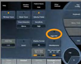
**High PRF** allows you to measure flows of higher velocities than those that can be measured with the maximum conventional available PRF, by increasing the PRF above the Nyquist limit and avoiding aliasing.
