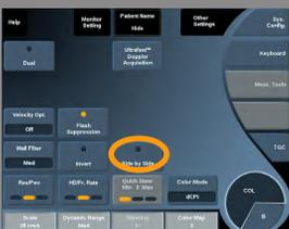
**Side by Side** allows you to split the screen in two live parts:
