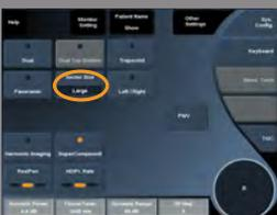
**Sector Size** widens or narrows the size of the sector angle to maximize the image's region of interest. Changing the sector size affects the frame rate. The narrower the sector size, the faster the frame rate.
