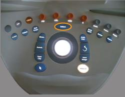
You can switch which of the dual images is active by pressing **Select**. Imaging settings will always be applied to the active image in dual. Imaging settings will be maintained independently for the dual images. If you press **Freeze** before **Select**, you can change image settings and modes on the active side.
