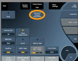
**UltraFast™ Doppler Acquisition** launches a 2-second prospective capture of CFI, CPI or dCPI at high frame rates.
