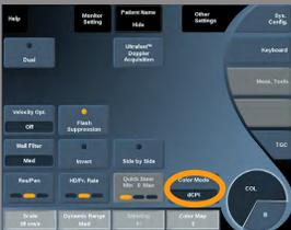
**Color Mode** allows you to switch between CFI, dCPI and CPI.
