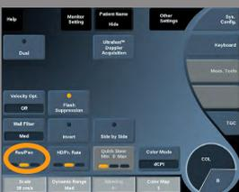
**Res/Pen** allows you to change the center frequency to reach increased resolution or increased penetration.
