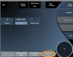
**SuperRes™** is an image processing feature which reduces speckle, improves image texture and enhances borders without an impact on frame rate.
