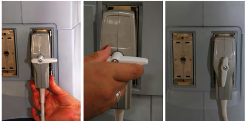
When disconnecting the transducer, turn the lock handle counterclockwise to unlock the connector and then hold the connector and pull it straight out.
