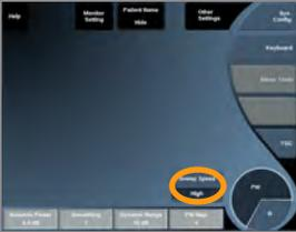
**Sweep Speed** allows you to change the speed with which the spectral columns are updated on the display.
