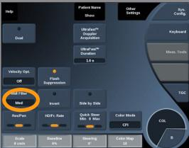
This parameter filters out low velocity signals. It helps to decrease motion artifacts caused by patient or transducer motion. **Wall Filter** is available only in live imaging. Touch **Wall Filter** until you select the desired value.
