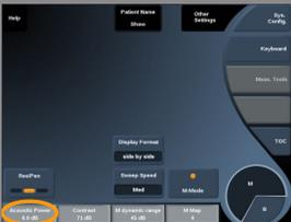
**Acoustic Power** indicates the output acoustic power. **Acoustic Power** is available only in live mode.
