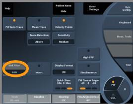
This parameter filters out low velocity signals.
