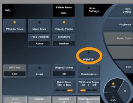
Press **PW Autotrace** to display the envelope of the peak velocity of the flow as a function of time.
