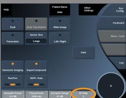
**2D Map** assigns the display of echo amplitudes to a range of grayscale or chromatic colors.
