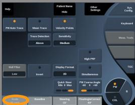
**Scale** allows you to modify the maximum velocities displayed on the Doppler spectrum.
