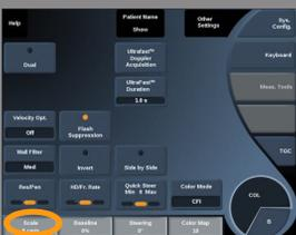
**Scale** allows you to adjust the maximum displayed velocity.
