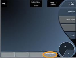
**Smoothing** is a spatial filter used to smooth the M-mode in order to provide a more homogeneous appearance.
