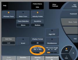
**Quick Steer** allows you to quickly steer the insonifying beam. Press **Quick Steer** to change its value. Use the **Steering** knob for finer settings.
