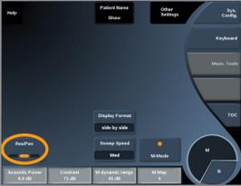
**Res/Pen** allows you to change center frequency to obtain increased resolution or increased penetration. **Res/Pen** is available only in live imaging. Press **Res/Pen** to change value.
