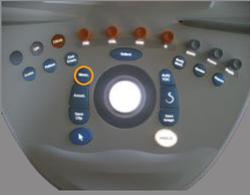
Press **Meas.** on the control panel to access measurements available in panoramic imaging.
