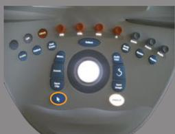
Press **Select** to change between **Box move** (position of the box) and **Box size** (resize the box).
