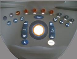
Move the **trackball** left and right to move the Doppler line in the 2D image.
