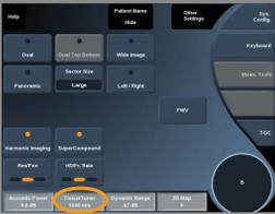
**TissueTuner™** allows you to adjust the receive parameters associated with the assumed speed of sound of ultrasound in the body. Adjusting the speed of sound parameter to match the type of tissue being interrogated results in increased spatial and lateral resolution.
