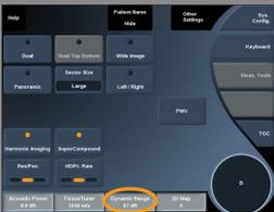
**Dynamic Range** Dynamic Range allows you to change the range over which the amplitudes of returning ultrasound signals are displayed.
