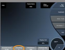
**Smoothing** is a spatial filter used to smooth the elasticity map in order to provide a more homogeneous appearance.
