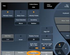
The insonifying beam can be steered in a direction as close as possible to the expected direction of motion, within limitations imposed by the transducer and the image plane geometry. **Steering** is available only in live imaging. Rotate the knob located under **Steering** to steer the Doppler line.
