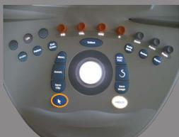
If several functions are available with the trackball, they are displayed at the bottom of the image. The active function is displayed in orange. Press the **Pointer** to change the active trackball function.
