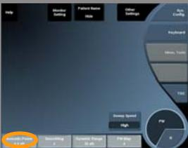
**Acoustic Power** indicates the output acoustic power.
