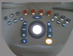
When in Live imaging, press **Freeze** on the control panel to freeze the image. A snowflake appears on the image to indicate the image is frozen.
