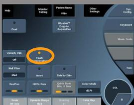
**Flash Suppression** utilizes an adaptive wall filtering scheme in order to suppress the flash artifacts due to tissue motion.
