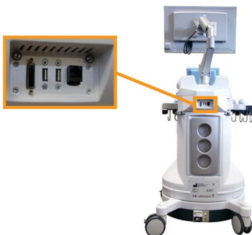
An external monitor which supports DVI capability may be connected to this port.
