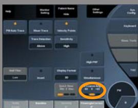
**PW Coarse Angle** is available in live imaging and on a frozen image. PW Coarse Angle is available in live mode only. Touch **PW Coarse Angle** until you select the desired value.
