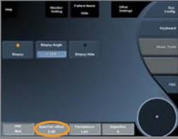
**AutoTGC offset** allows you to program automatic overall gain when using the **AutoTGC**.
