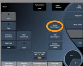
This control deletes the active spectrogram and corresponding sample volume from the image.
