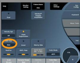
This parameter filters out low velocity signals. It helps reduce motion artifacts caused from breathing and other patient motion. **Wall Filter** is available only in live imaging. Touch **Wall Filter** until you select the desired value.
