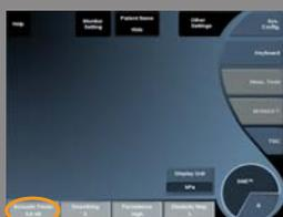
**Acoustic Power** indicates the output acoustic power.
