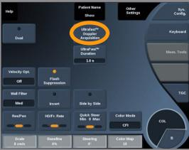
**UltraFast™ Doppler Acquisition** launches a prospective capture of CFI, CPI or dCPI at high frame rates.
