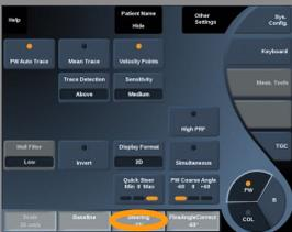
The insonifying beam can be steered in a direction as close as possible to the expected direction of motion, within limitations imposed by the transducer and the image plane geometry.
