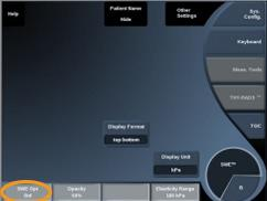
**SWE Opt** allows you to optimize the elastography resolution and penetration according to the area you are scanning.
