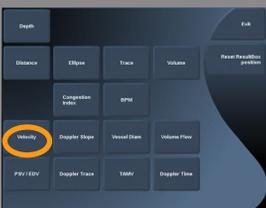
The **Velocity** tool results in a Doppler Velocity (Vel) measurement (in cm/s) and a Pressure Gradient (PG) calculation (in mmHg).
