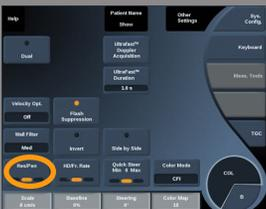
**Res/Pen** allows you to change the center frequency to reach increased resolution or increased penetration.
