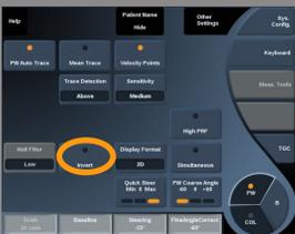
**Invert** vertically flips the spectral display without affecting the baseline position.
