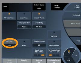
This parameter filters out low velocity signals.
