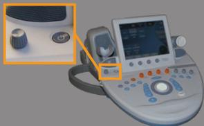
1. Press the **On/Off** button on the control panel, next to the left speaker. The system automatically checks a certain number of components and peripherals and boots up.
